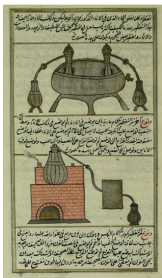
Fig. 1 Two different distillation processes are depicted in Salih b. Nasrullah's Ghayat al-itqan fi tadbir badan al-insan (The highest perfection in the treatment of the human body) written in Arabic. The copying date is 1722). The figure above illustrates a process in a sand bath, while the one below shows a process using a briquette oven. Süleymaniye Library (Istanbul) MS Ayasofya 3682, 26a.
